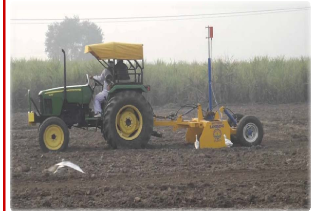
Figure 3: Bucket leveler with laser attachment, Hydraulically operated drag buckets
