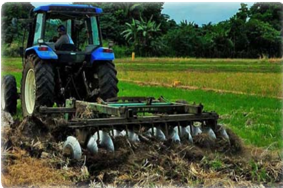
Figure 1: Primary Land Tillage using Disc Plough
